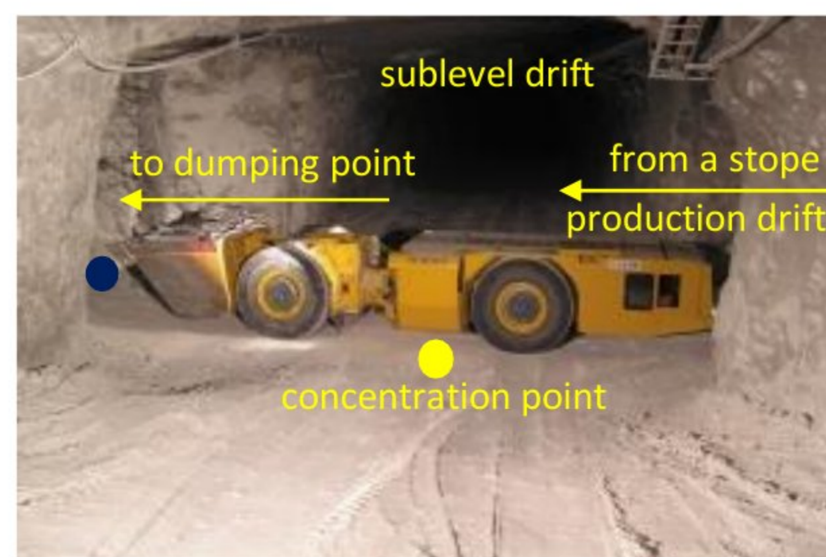
Figure 7. Load–haul–dump (LHD) vehicle in operation on sublevel; figure adopted from [31] and transformed.
