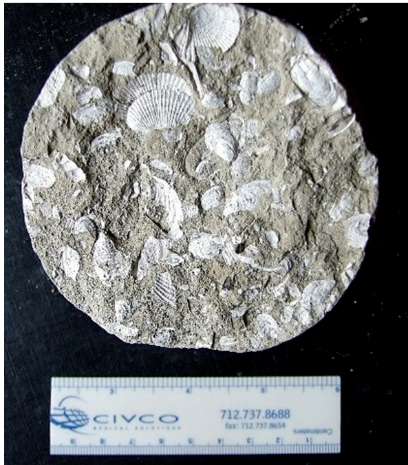
Fig. 9. Pannonian marl with Congeria banatica R. Hoernes and other mollusks (SA-2, 55 m). Photo by Lj. Rundić
