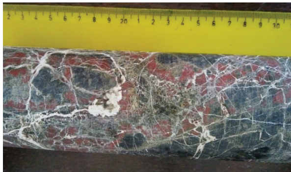
Fig. 5. Detail of hard, reddish-gray and dark green conгло-breccia probably of the Lower Cretaceous. Borehole SA-2 (334 m). Photo by Lj. Rundić
