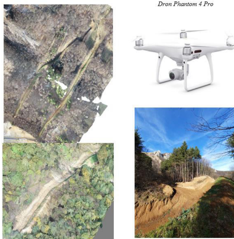
Figure 1. Orthophoto shot of the protective channels at the foot of the Starica mountain (shot from a drone) and a picture of the channel from the field
