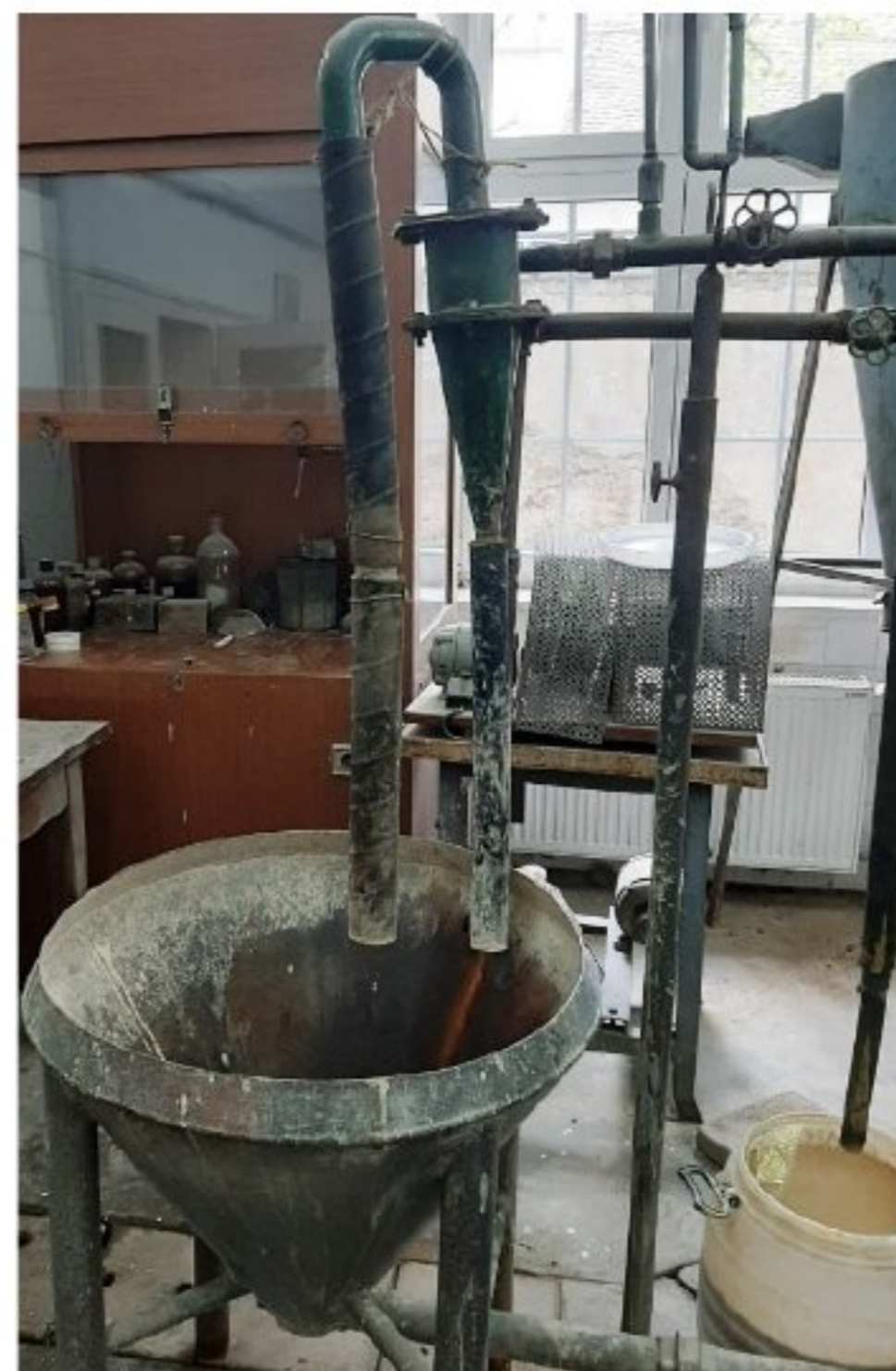
Figure 6 Laboratory setup for hydrocyclone testing
