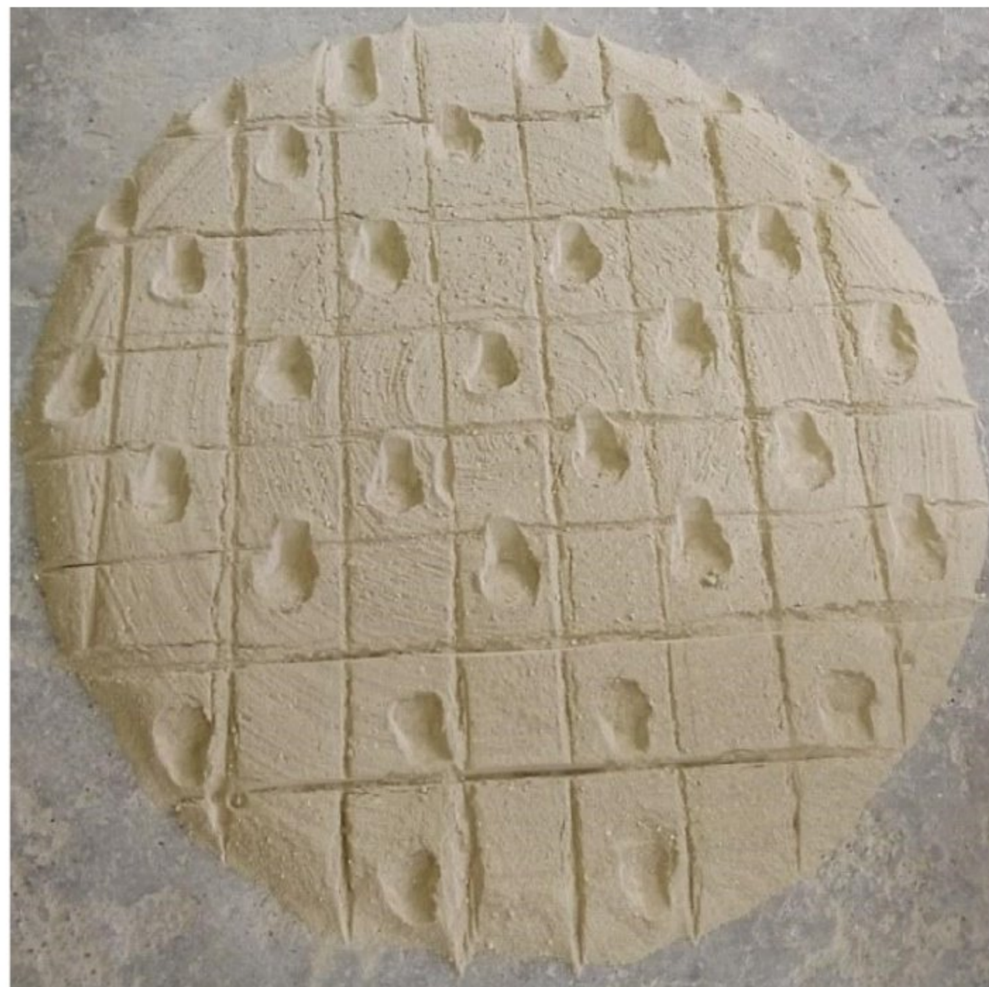
Figure 2 Cake after sampling using the checkerboard method
