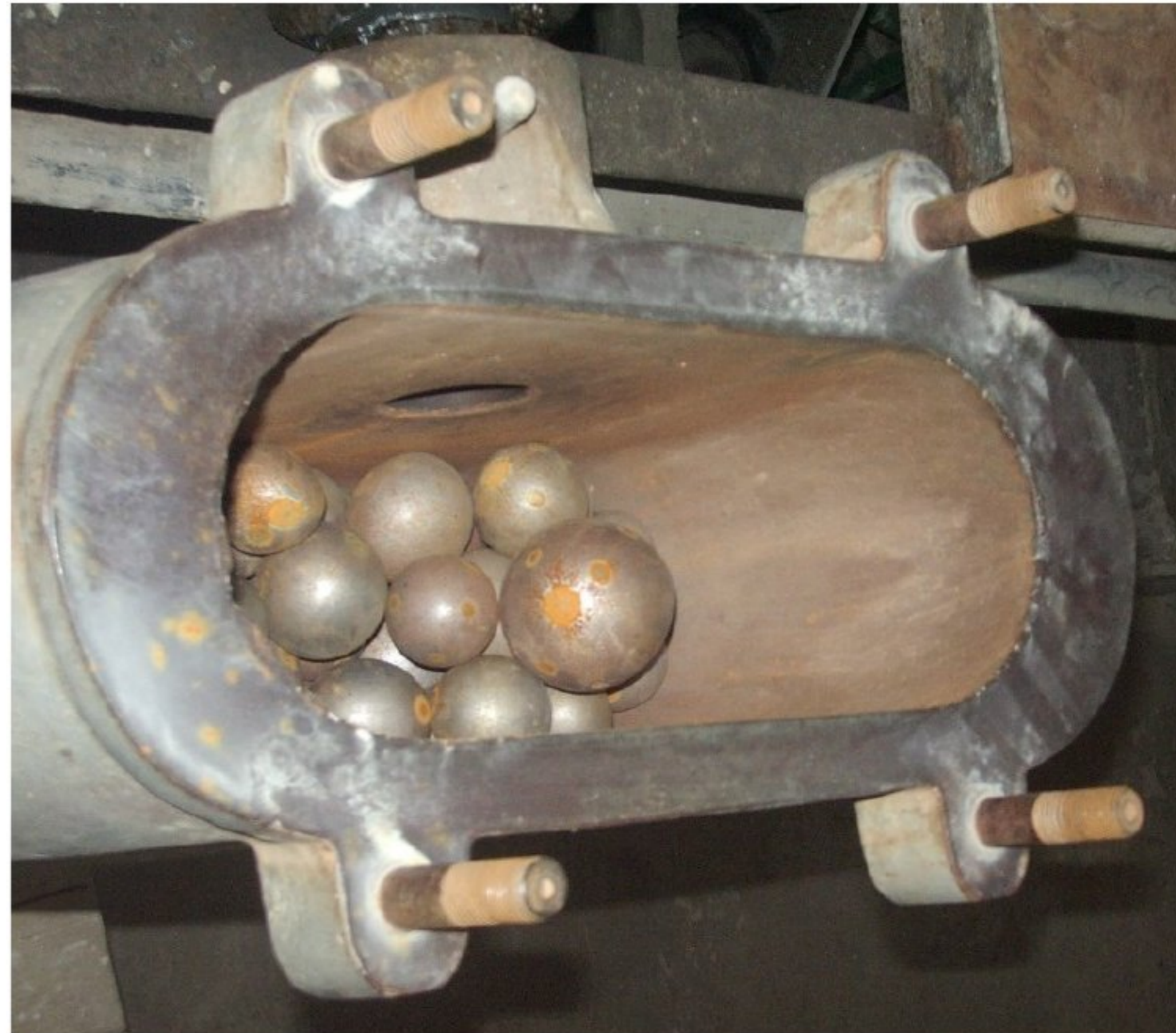
Figure 4 Denver laboratory mill (Deušić & Lazić, 2013)
