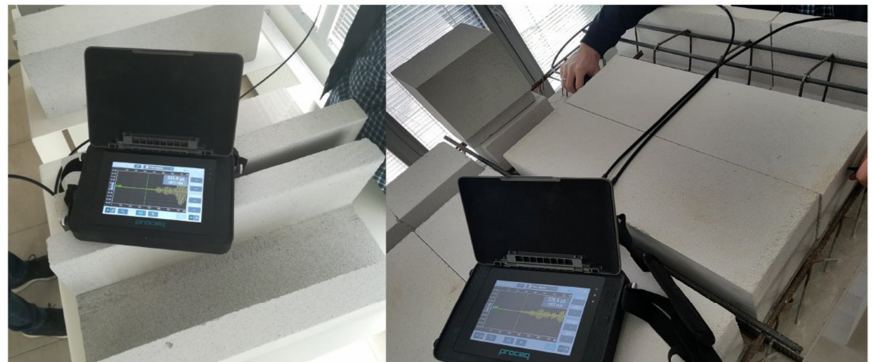
Figure 4. Instrument and display used in the measurement with the speed of longitudinal waves on blocks.
