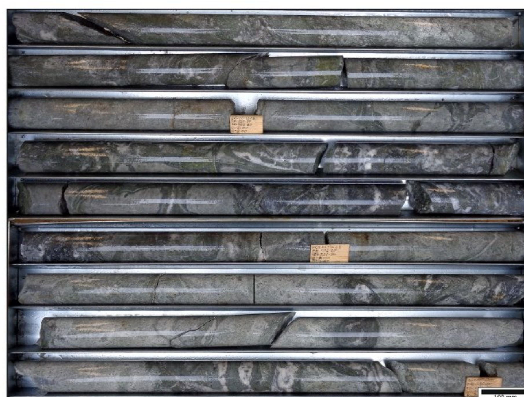
Fig. 5. Example drill core of the shallow igneous breccia unit at the base of the volcanic stack, hosting clasts of mineralized skarn set within an igneous-hydrothermal matrix. Image is of drill core EOKSC1678, from the core depth 231.6 to 240.9 m.
