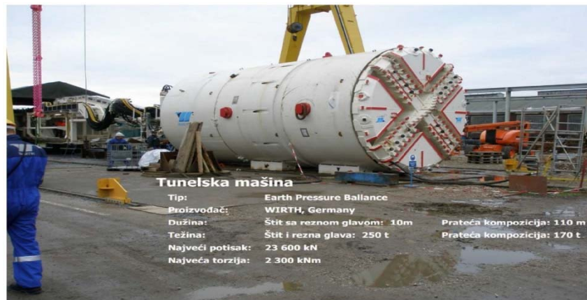
Slika 46. Tunelska mašina Earth Pressure Balance (Institut Jaroslav Čemir AD, 2009)
