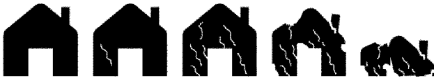
Fig. 3 Typology of most common object damage classification: negligible; negligible to slight; moderate; prone to collapse; destroyed
