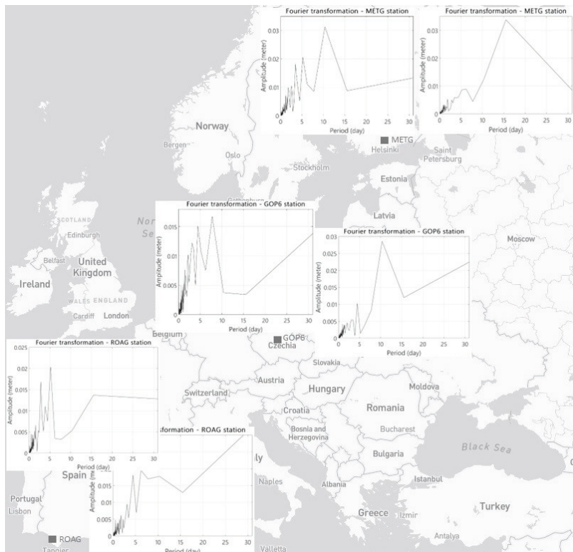
Figure 1. Spatial distribution and corresponding FFT of ZTD of IGS stations METG, GOP6, ROAG for July 2022 (left) and January 2023 (right).
