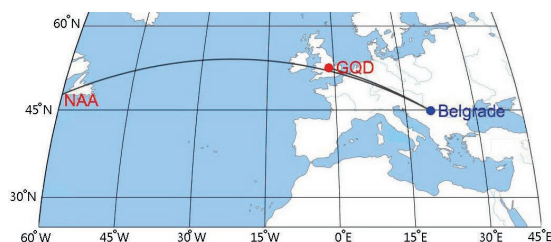
Figure 1. Map with analysed VLF signals' GCPs (black lines) emitted towards BEL receiver site (blue circle) from USA (NAA/24.0 kHz) and UK (GQD/22.1 kHz) (red circle).
