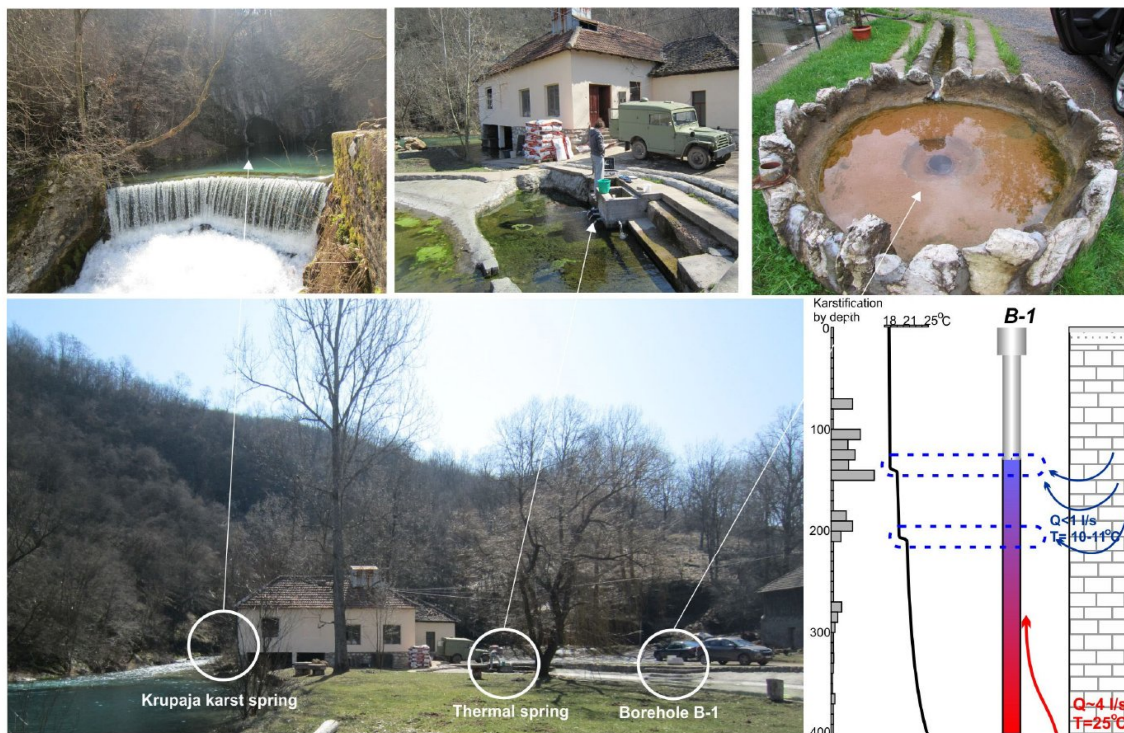
Figure 3. Krupaja system phenomena (Krupaja Spring, thermal spring, and borehole B-1). Borehole B-1 log according to video-endoscopy, thermal logging, and flow meter logging data.
